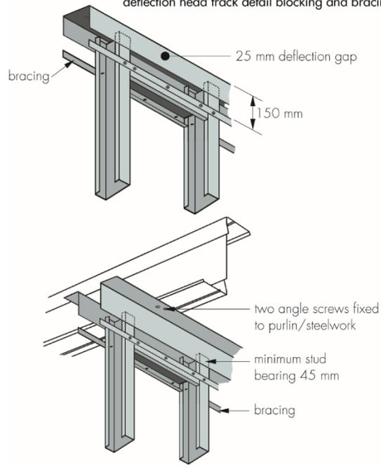
lateral restraint blocking and bracing
