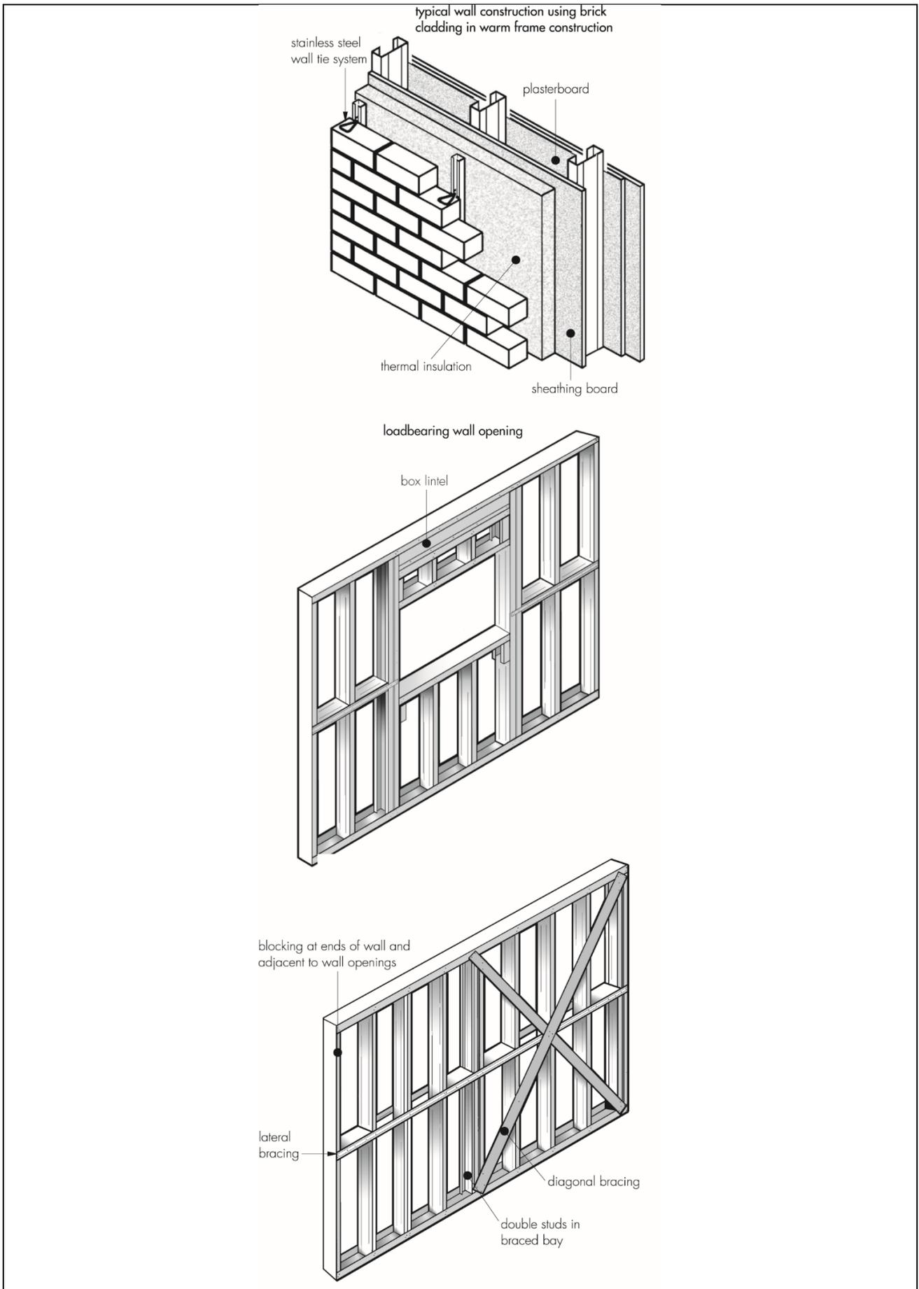
Figure 7 Typical detail partition wall
