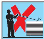
Wherever possible lift sheets manually onto the roof. Where they have to be hoisted into position make sure the edges are protected and pressure across the sheet does not cause distortion. Use only ropes or slings for hoisting, never use chains.
